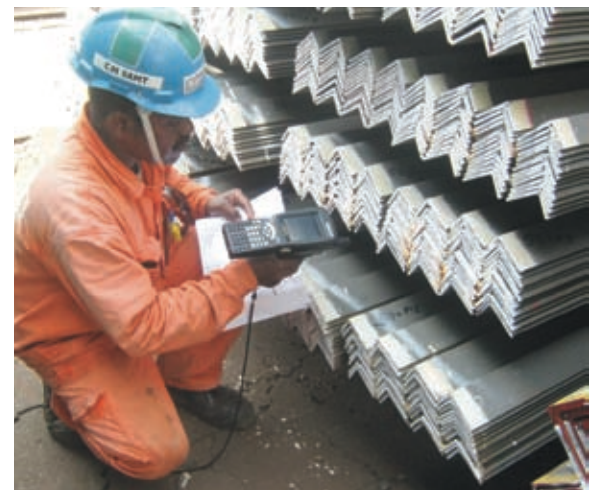
Keppel FELS has developed and implemented bar-coding system to save costs
