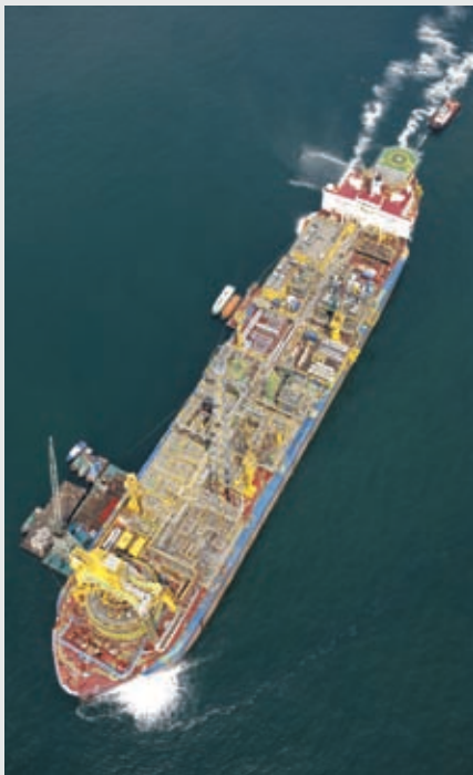
Operating in the Campos Basin of offshore Brazil, Espirito Santo is the first turret moored FPSO in the world using steel catenary risers for fluid transfer.
