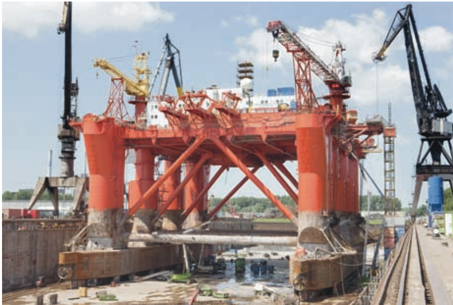
COSLRIVAL, an accommodation semisubmersible being repaired and upgraded in Keppel Verolme's dry dock
