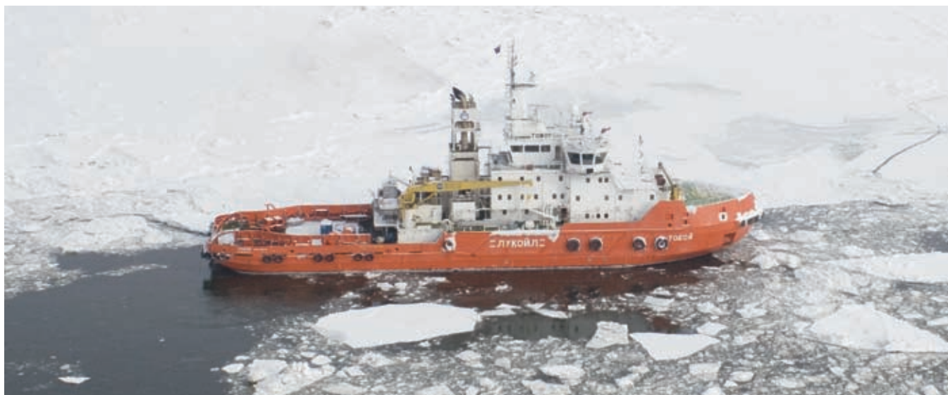
Slicing through ice sheets of up to 1.4m thick, Toboy surmounted the rigorous tests in the Kara Sea
