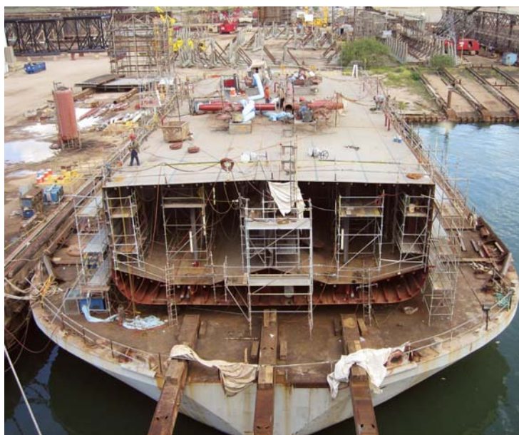
Right: Measuring 150,000 cubic feet, Red Hook is a custom-built sludge vessel for New York City
