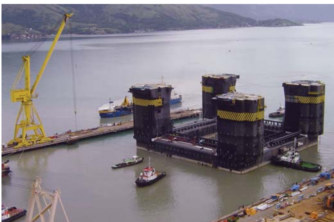
Three months after her arrival (left), the P-52 lower hull was anchored and submerged on location, in anticipation of the mating with the upper hull
