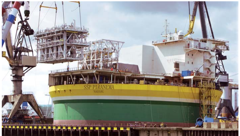
The round-shaped FPSO Piranema resting inside Keppel Verolme’s mammoth drydock for commencement of its survey works and heavy lifting activities
