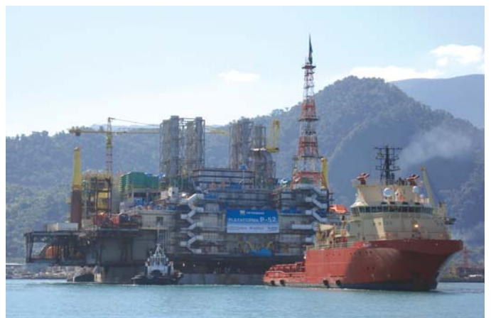
Three months after her arrival (left), the P-52 lower hull was anchored and submerged on location, in anticipation of the mating with the upper hull
