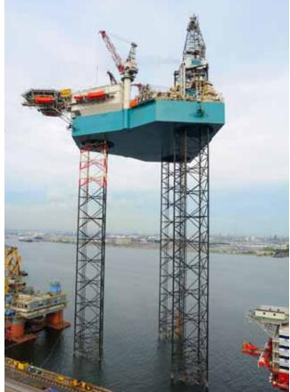
Keppel has delivered to Rowan companies three KFELS N Class jackups. The design is in full compliance with requirements for rigs operating in the Norwegian sector of the North Sea
