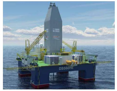
Equipped with winterised features such as derrick cladding and machinery space heating, DSS<sup>TM</sup>51HE and DSS<sup>TM</sup>60HE (pictured) semis are capable of year-round operations
